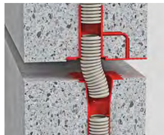
Compensation in transverse direction \pm 10 mm.
