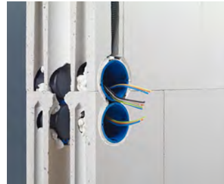
Cables up to Ø 11.5 mm and conduits up to M25 can be fed into the sound insulation box.
