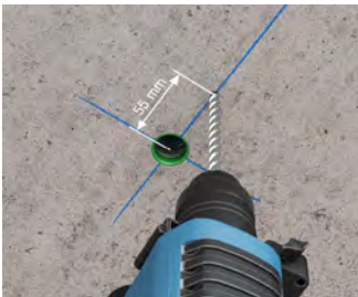
Drill a Ø 8 mm hole for a standard dowel and insert the dowel.
