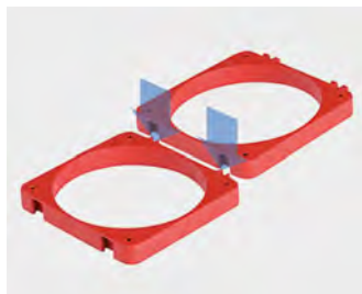
For combinations position the centering aid at a distance of 71 mm.
