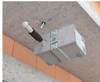
Break out the conduit entry or cut an exact cable entry for airtight installation, e.g. by using the KAISER universal opening cutter (Art. No. 1085-80).
