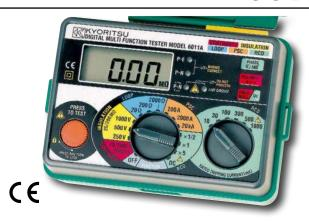
The Model 6011A can perform FIVE separate test functions: insulation, continuity, earth loop impedance, prospective short circuit current and RCD trip testing in full compliance with IEC 61557.
