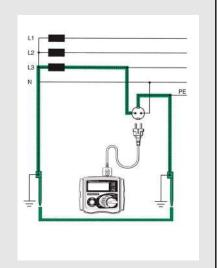
Fig. Earth fault loop impedance testing at socket outlet.
