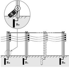
Rx, is defined as earth resistance under test, and R1, R2...Rn are defined as earth resistance of other measuring objects.
