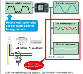
Unlike to traditional measuring apparatus, less susceptible to narmonics noises. Successfully achieving logging with no effects of harmonics by True RMS calculation every 200 ms using FFT (Fast Fourier Transform).
