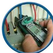
KEW FORK 2300R can be used in crowded connection boxes, where cables are very short, and space is too limited to clamp cables using with a traditional clamp meter.
