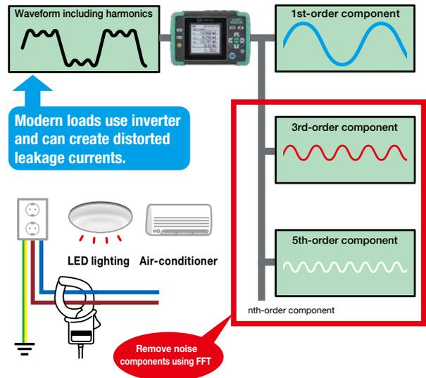
Unlike to traditional measuring apparatus, less susceptible to harmonics noises. Successfully achieving logging with no effects of harmonics by True RMS calculation every 200 ms using FFT (Fast Fourier Transform).
