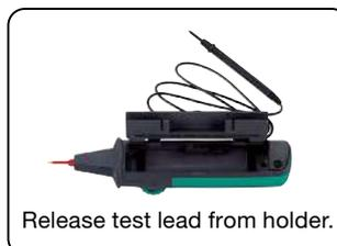
Release test lead from holder.
