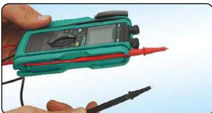
Test Probe can be fixed to the holster
