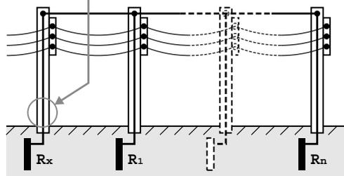
$R_x$  is defined as earth resistance under test, and  $R_1, R_2, \dots, R_n$  are defined as earth resistance of other measuring objects.
