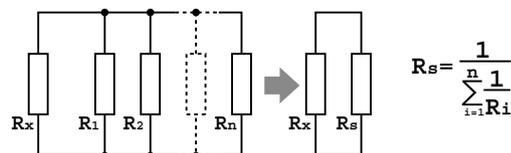
Voltage  $V$  is applied to the object (Resistance  $R_x$ ) measured from the voltage injection transformer CT1, and the current  $I$  corresponding to the earth resistance is flowed.
